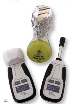
excitation, i.e., for measuring chlorophyll fluorescence in algal cultures. Red-orange excitation light (620 nm) is intended for excitation through phycobilins and is suitable for measuring in cyanobacterial cultures.
