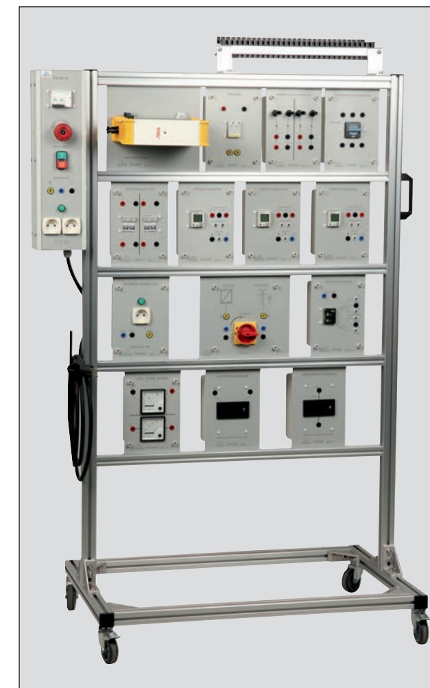
Set of photovoltaic modules (H-250mm) and solar panels for studying a solar installation with energy feeding to the 230V AC grid.
