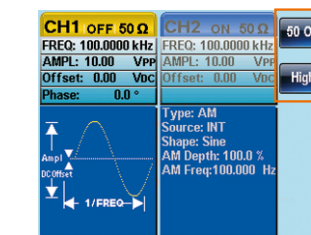
50Ω / High Z Impedance Switch Function
