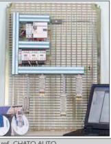
Wired door plate and grid for system operation with a Twido PLC. Supplied with programming and training software
