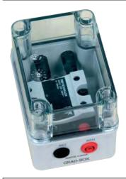
Controls the power in the charge by varying the conduction angle of the thyristors according to the control current of 4-20mA. Can be connected directly to the built-in PLC unit ref. AUTO-BOX-A.
