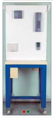
GES-7 is a programming and wiring panel for a BUS wired (two wires) anti-intrusion alarm unit. This unit monitors two areas in the business premises by means of a passive infrared sensor, a dual-technology intrusion sensor (infrared + microwave frequency) and two magnetic sensors which are triggered if the windows are opened. A keypad for entry code, which is built into the unit, activates or deactivates monitoring of the area.
