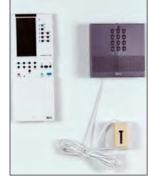
This panel presents the home automation management of energy saving functions by using electric management modules. It uses modern products such as pilot wire heating, control of roller-blinds, a power manager, a load shedding function and remote control via a telephone.
