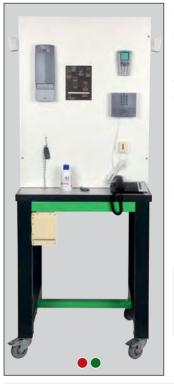
GES-92 is a panel used for studying and programming a wireless anti-intrusion alarm unit with a built-in siren. The unit is fitted with 2 passive infrared sensors and a magnetic sensor which is triggered if the window is opened. The keypad for code entry enables or disables the alarm remotely. A transmitter associated with an automatic switchboard reports any triggering of the alarm via a remote telephone. The transmitter is easy to program, thanks to its built-in keypad.
