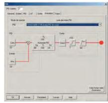
PID function from the PLC. The values of the settings, temperature, power output and the proportional and derived coefficients are completely configurable.
