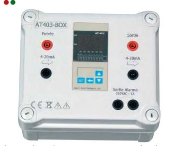
The PID regulator is the correcting component into a regulation loop for the monitoring of a process (boiler, compressor, pump ...). It receives a 4-20mA signal from the sensor which is the image of the value to regulate (temperature, pressure, flow...). It compares it to the set-point (programmed in the PID) and drive the process to reduce the difference "process variable / set-point"
