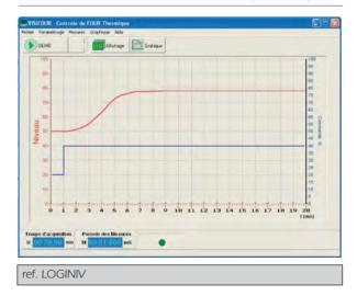
This PC interface – connected to the DB9 outlet – and software are used to record and draw graphs of instantaneous water level and control signal of the pump speed directly on PC. The connection to PC is made by USB.
