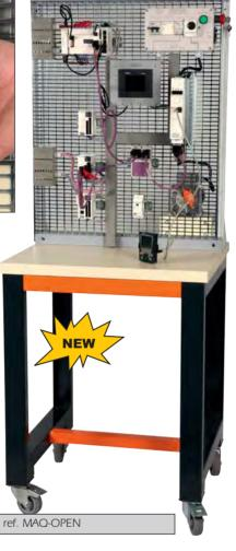
MAQ-OPEN includes Schneider® components and enables study of the Modbus Series, CANopen and Ethernet buses.
