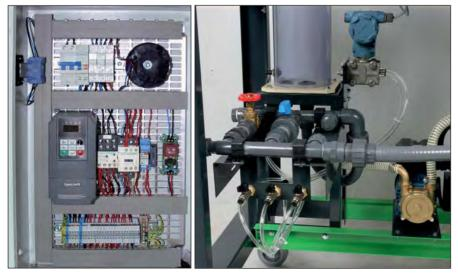
Wired grid including with a speed controller
