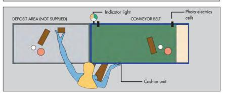
TAPIX is a conveyor belt for a cash register with the same features as the ones you would find in a supermarket. It comprises a conveyor belt driven by a gear motor, a control unit used by the cashier, an indicator light showing the status of the cash till and start and end of belt sensors. Two TAPIX models are available:
