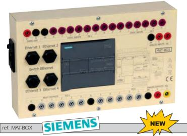
MAT-BOX is a SIEMENS® SIMATIC S7-1200 PLC unit fitted with safety terminals 4mm to facilitate the connection of sensors and other actuators. The integral PROFINET interface ensures communication simplicity for programming, link to the HMIs and CPU-to-CPU dialogue.
