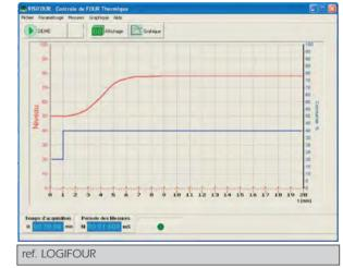
This PC interface – connected to the DB9 outlet – and software are used to record and draw graphs of temperature and heating control directly on PC. The connection to PC is made by USB. ADDITIONAL FUNCTIONS
