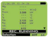
Measuring system efficiency
