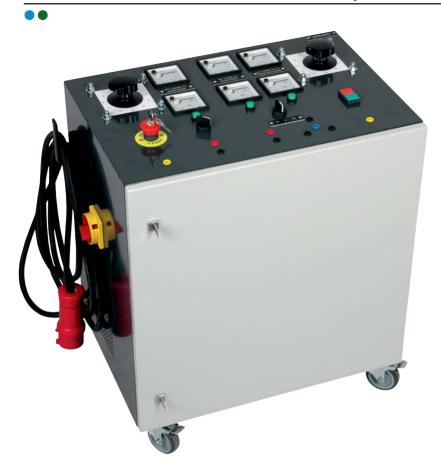
Transportable variable supplies unit (2000W or 4000W) Supply from mains: 3-phase 380V/400V + neutral + earth Outputs: 2 variable DC supplies 0-250V and 1 variable AC 3-phase supply 0-430V
