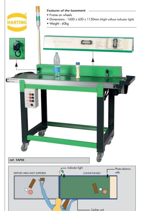
TAPIX is a conveyor belt for a cash register with the same features as the ones you would find in a supermarket. It comprises a conveyor belt driven by a gear motor, a control unit used by the cashier, an indicator light showing the status of the cash till and start and end of belt sensors.
